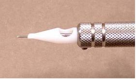
Picture on the left shows a short *Tip off* distance and the right shows a long Tip off distance. A long Tip off will allow the user to see more of the needle while running, but will not draw as much pigment from the tube as a short Tip off.
